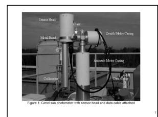
We need to give input to the Sunphotometer the exact latitude and longitude and also the GMT of the sampling location. Then it starts measuring from sun rise to sunset.
